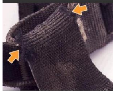
Beginning of a break at crossing point
